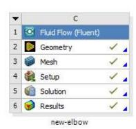
b. Select the **Solution** cell in the second Fluid Flow analysis system (cell B5) and drag it over the **Results** cell in the **Results** system (cell C2). This creates a transfer data connection between the two systems.
