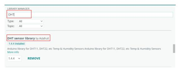
After installing the DHT library from Adafruit, type "**Adafruit Unified Sensor**" in the search box. Scroll all the way down to find the library and install it.
